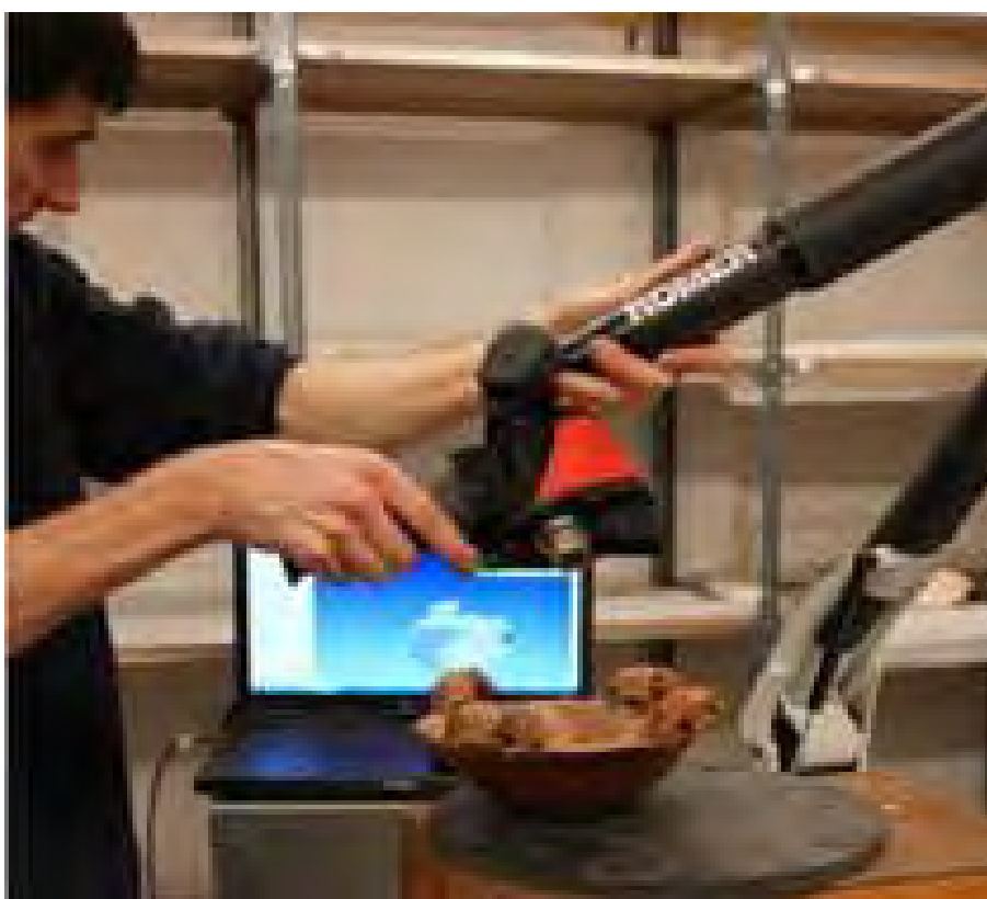
Fig. 4. Presynaptic hippo bowl being laser scanned for inclusion in the Haptic interface.
